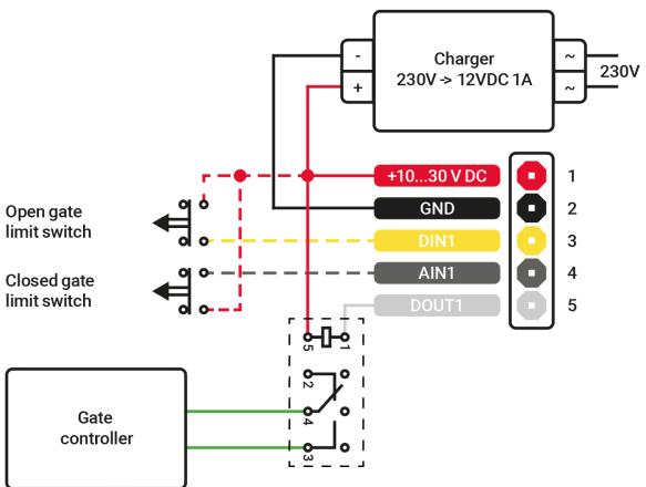
In the case of gate control only, it is required to connect the relay shown in the diagram above (not included in the set).
