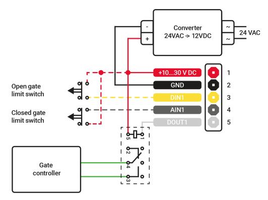
Before connecting the converter, make sure that the available power supply for the accessories in the gateway has the appropriate current capacity for the FMC920 and the gate control relay. The dotted lines indicate the possibility of obtaining optional information about the position of the gate (open, moving and closed) - this option requires additional limit switches that are not included in the set.
